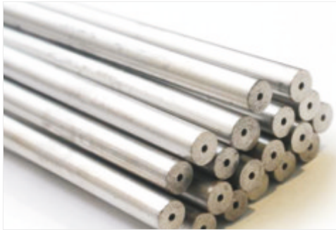
Carbide Rods with single hole Standard grades : BT10 and BT10X Submicron grain size, with all HIP treatment
