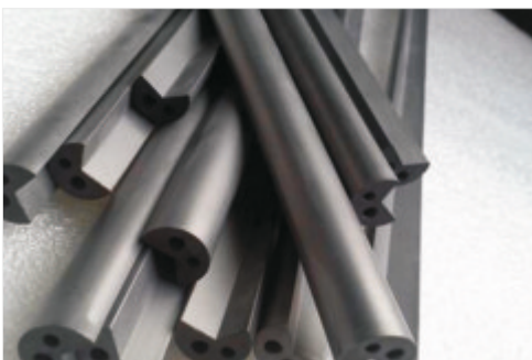
Blanks with round & kidney shaped coolant ducts Standard Grades : BT10 / BT10X Submicron grain size, with all HIP treatment.
